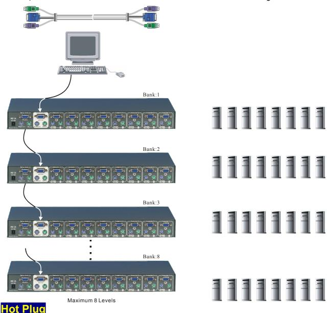
The KVM Switch supports "Hot Plug" function for easy addition or removal of PCs. The user can arrange or maintain PCs as follows:
